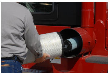
Donaldson Air Cleaner with Safety Element (Standard)
