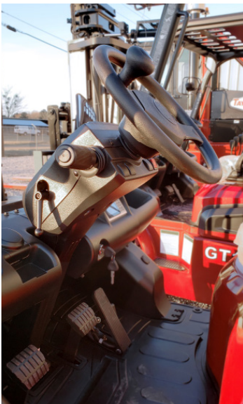
Adjustable Steering Column Pivots 30 Degrees
