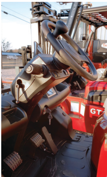
Adjustable Steering Column Pivots 30 Degrees
